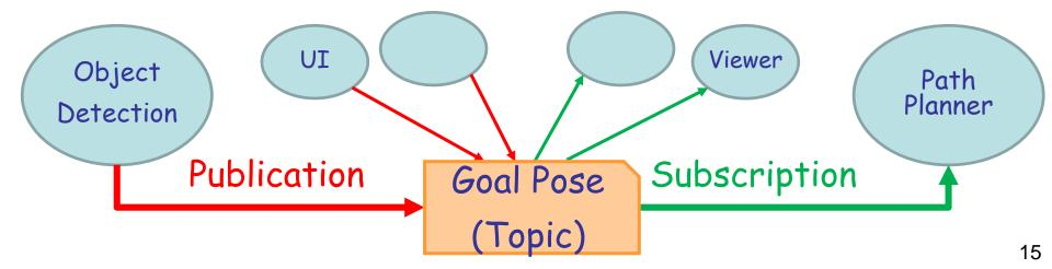
**Message**: Strictly typed data structure used for communication between nodes
